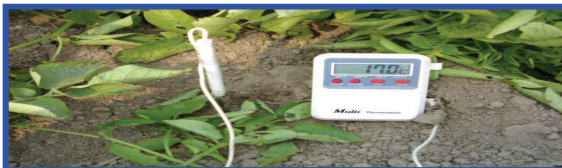
Photo 2. Recording of Soil temperature by digital soil thermometer
