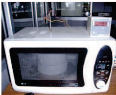
Figure I : Microwave furnace; Figure II: Schematic display of the sintering packet; 1. Aluminium plate; 2. Zirconia cylinder; 3. Samples; Thermocouple; 5. Al-25/1700 insulator; 7. SiC rods; 7. Microwave port; Figure III: Insulating packet in Microwave Furnace in microwave processing
