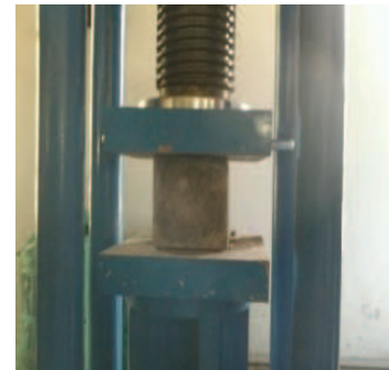
(c) Testing of Cubes
